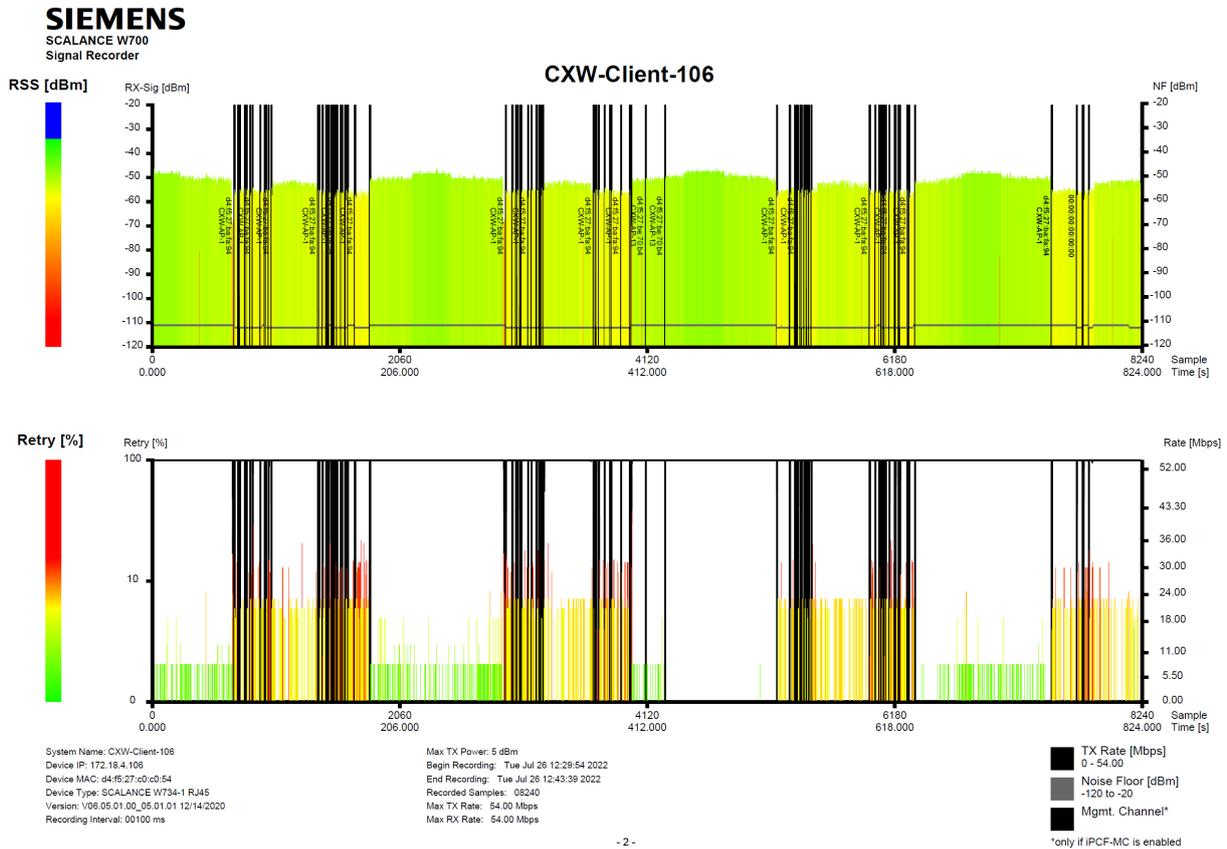
Fig. 202: Multiple crossing of same segment transfer with incorrect roaming processes (multiple vertical black lines in transfer area)
