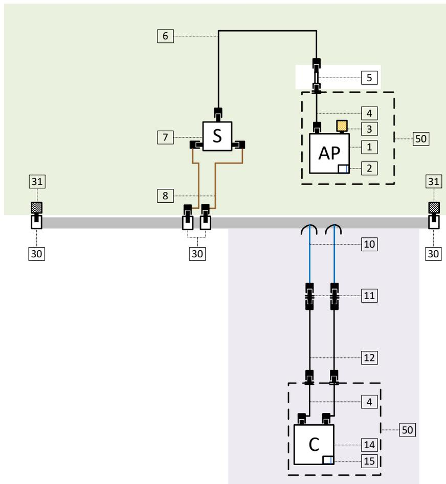
Fig. 29: Overview and arrangement of electrical components. Example: Line feed, client with two antennas, without additional housing, equipotential bonding not shown
