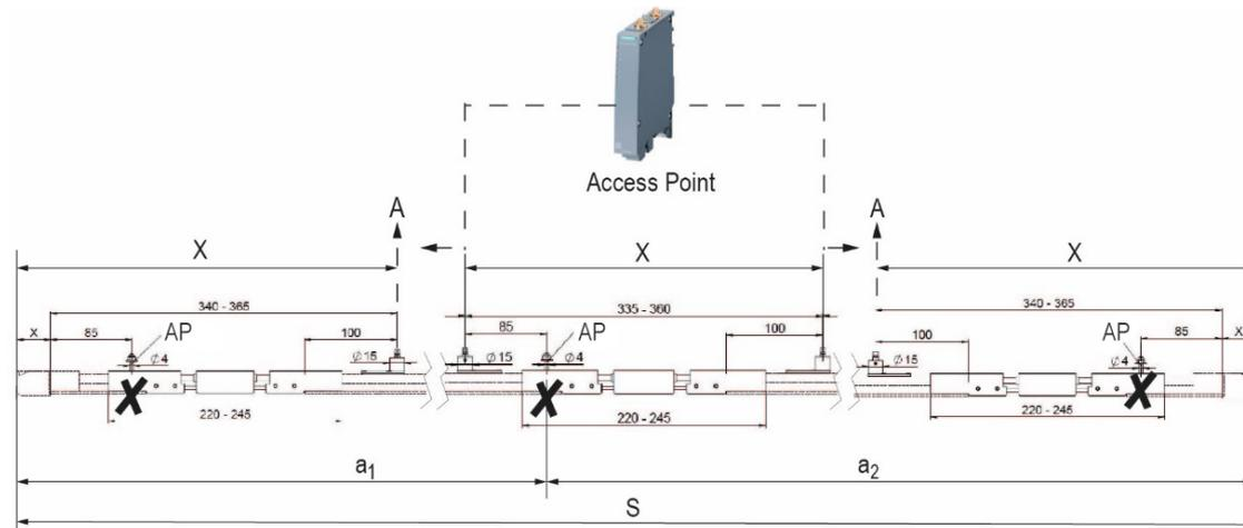
Fig. 51: Expansion unit dimensioning on segment
