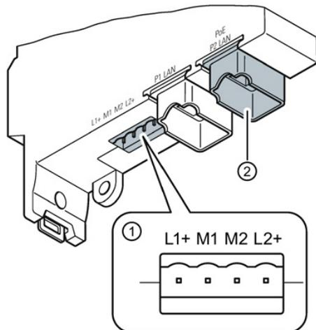
Fig. 145: Transceiver connection for Ethernet
