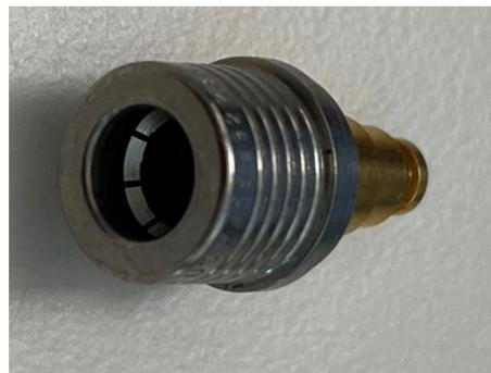
Fig. 14: QMA terminating resistor
