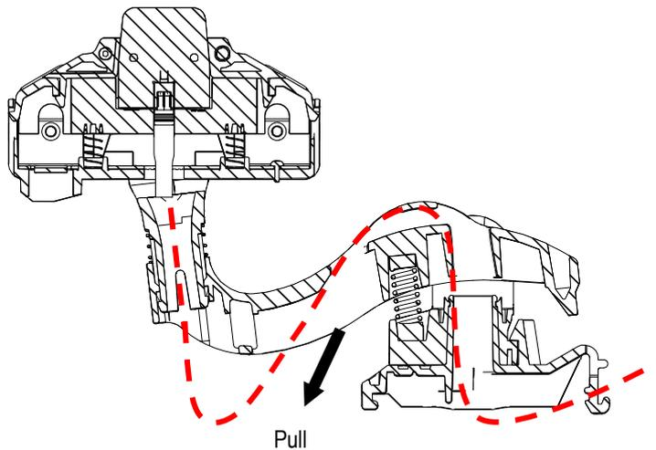
Fig. 172: Pull data cable (HF cable) (loop from below)
