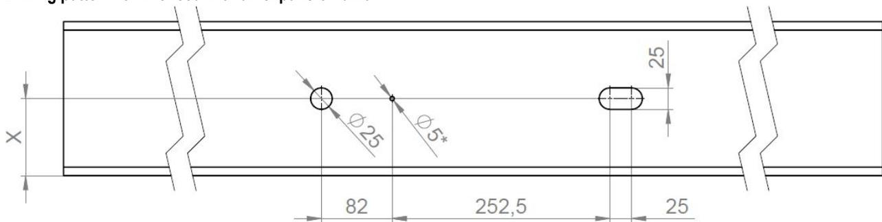
Fig. 119: Drill hole positions for line feeds with expansion unit and without overrun cap
