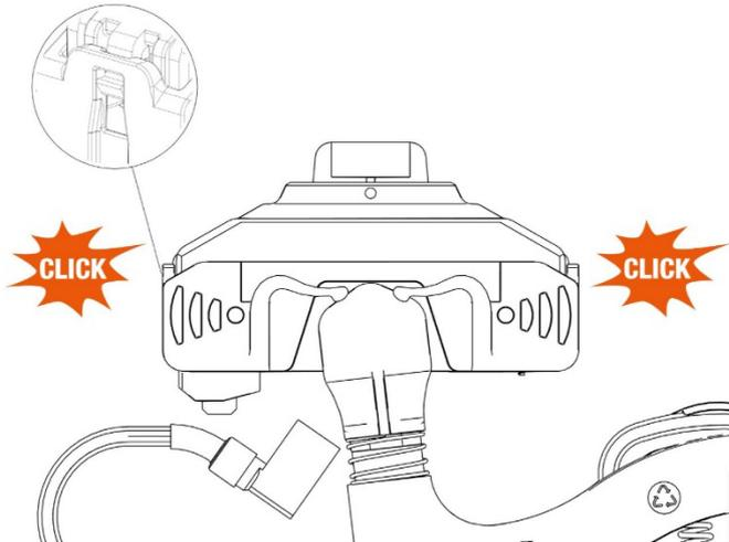
Fig. 169: Collector housing audibly clicks into place
