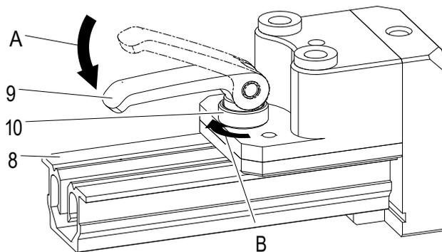
Fig. 109: Fix data rail in drilling jig
