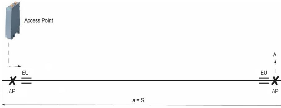
Fig. 52: Expansion unit layout at end
