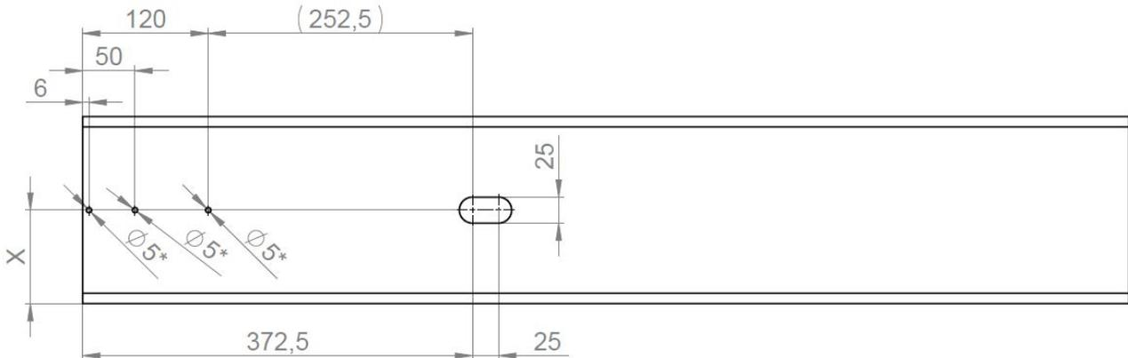
Fig. 121: Drill hole positions for end feed with expansion unit and plastic overrun cap
