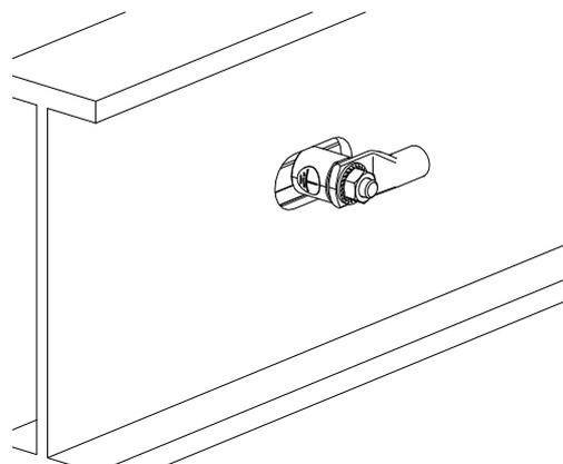
Fig. 85: PE connector seated in elongated hole
