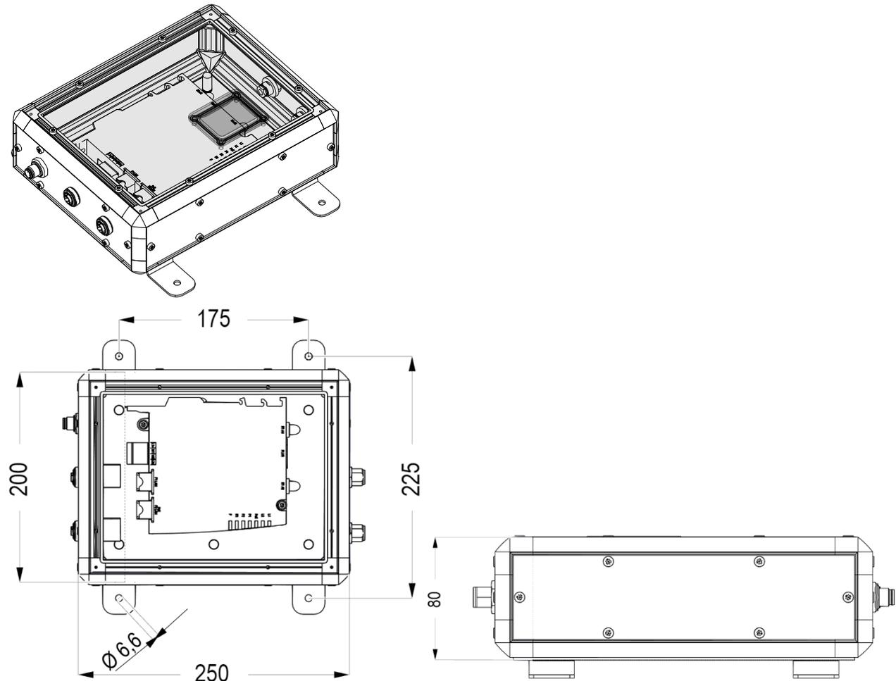
Fig. 3: Transceiver housing dimensions and illustration
