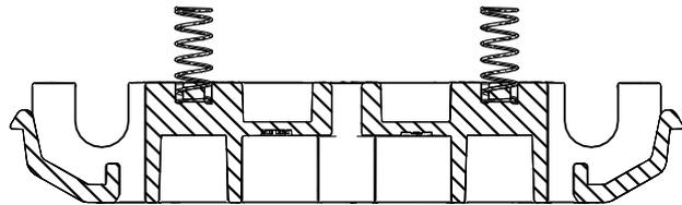
Fig. 156: Compression springs in centering
