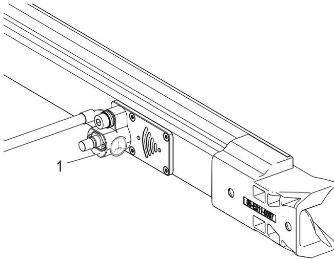
*Fig. 139: Line feed to stationary antenna*
