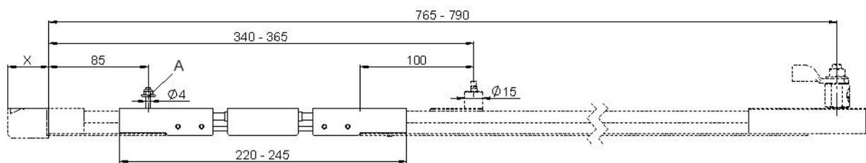
Fig. 66: Expansion unit – end feed (mounted on left), A = Anchor point
