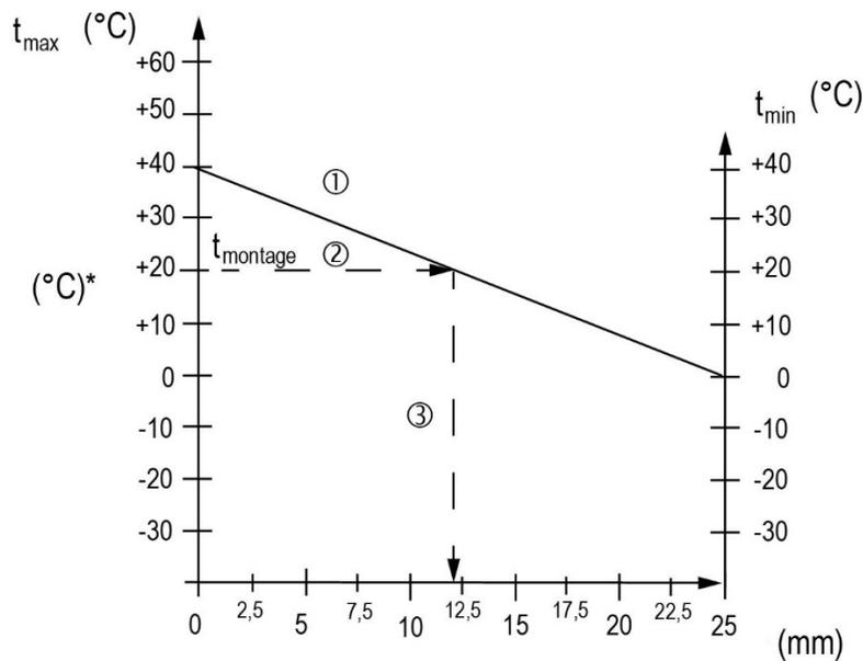
Fig. 55: Determine air gap
