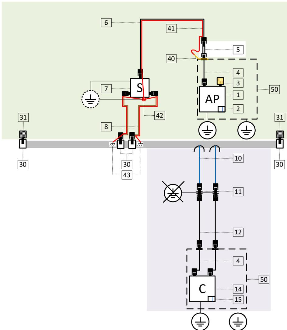
Fig. 138: Principle diagram of equipotential bonding (red) and grounding (symbol)
