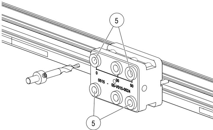
Fig. 91: Drill 4 holes for PE connector
