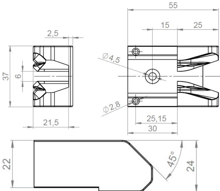
Fig. 118: Aluminium transfer guide
