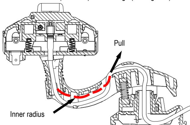
Fig. 184: Pull data cable back through (HF cable)
