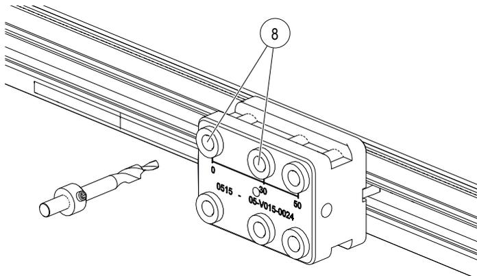
Fig. 94: Drill 2 holes for PE connection
