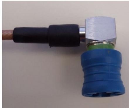
Fig. 7: QLS connector is locked (green ring visible by pushing the blue sleeve forward)
