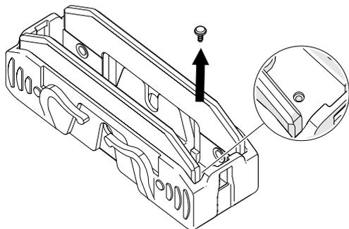
Fig. 158: Loosen STS-plus 1.4x4-T5 screw
