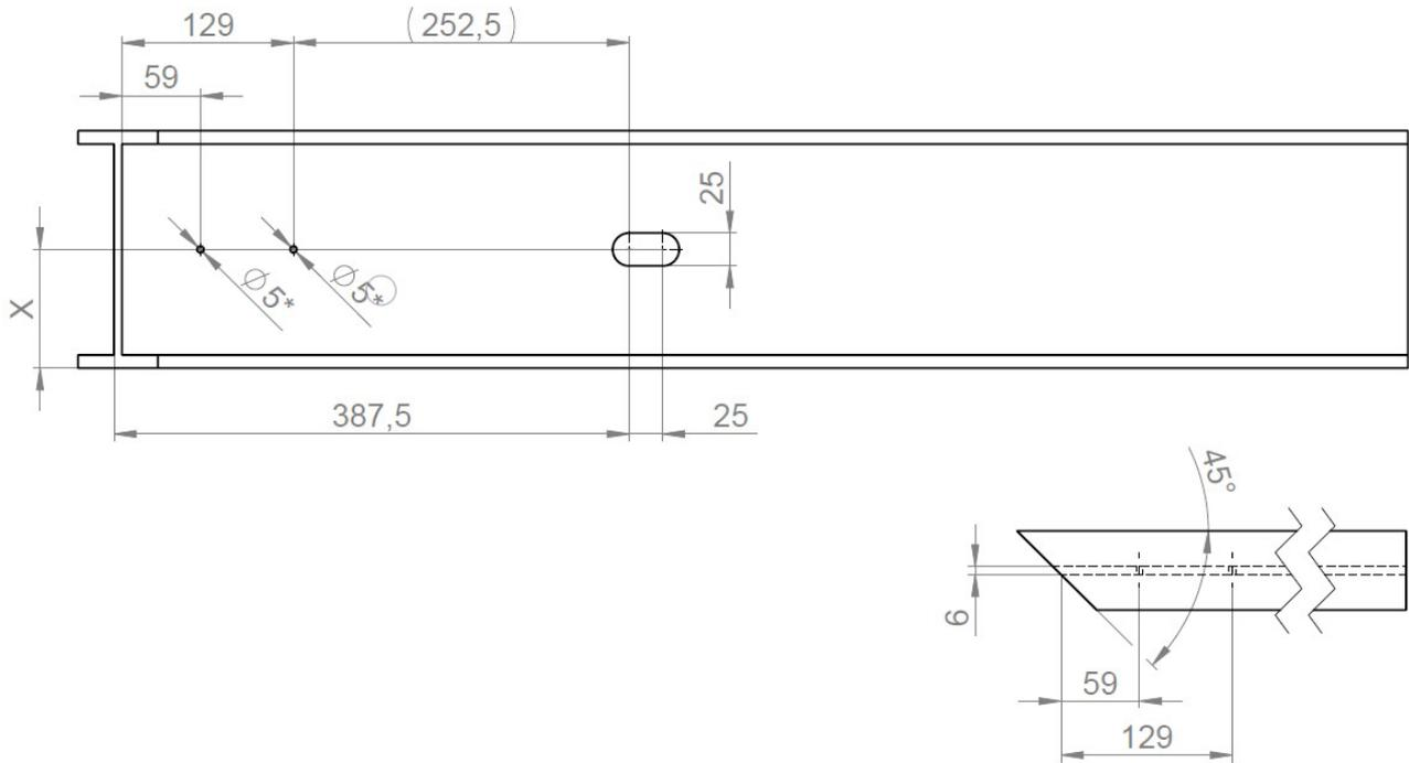
Fig. 123: Drill hole positions for end feed with single expansion unit with aluminium overrun cap (45° cut on long side of substructure (support structure))
