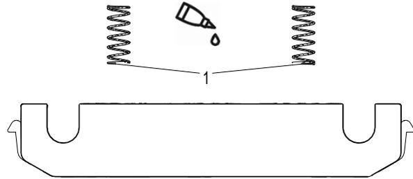
Fig. 155: Apply adhesive to first turn of spring
