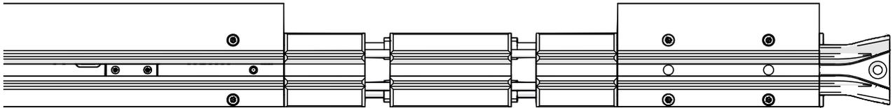
Fig. 69: Expansion unit – end feed (mounted on right)
