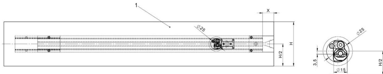
Fig. 48: Support structure (substructure) (1) with line feed (aluminium cap, right)
