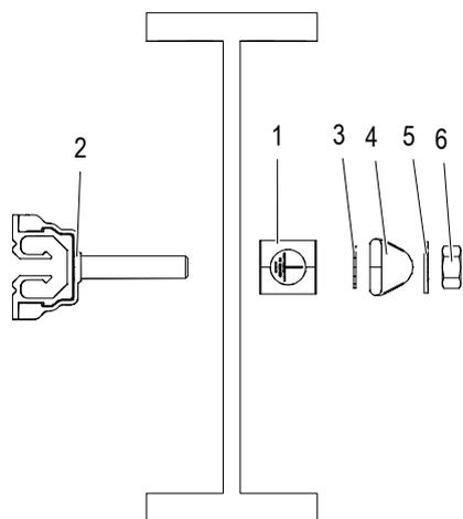
Fig. 84: Mount PE connector onto support structure (substructure)
