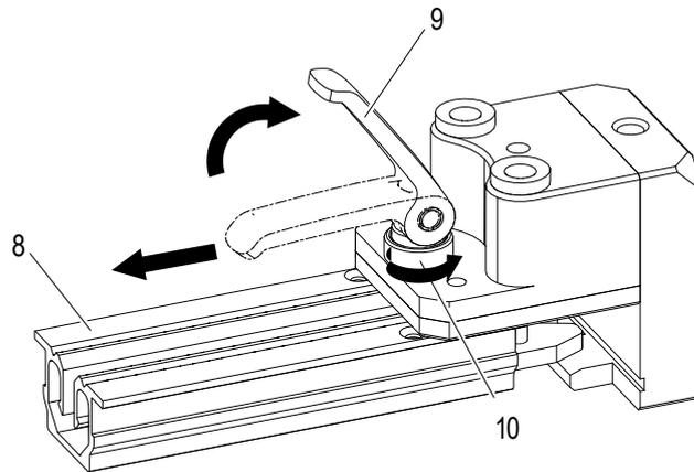
Fig. 112: Remove data rail
