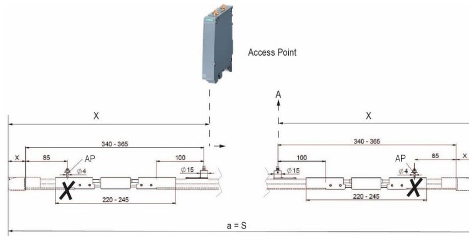
Fig. 53: Expansion unit layout at end
