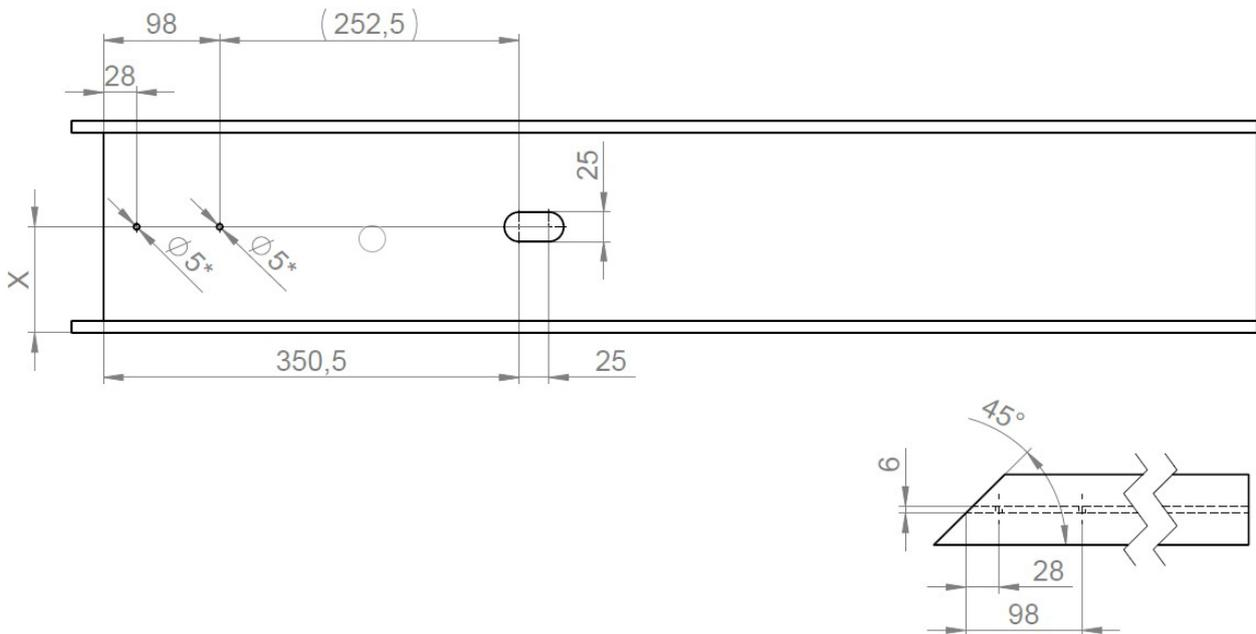
Fig. 122: Drill hole positions for end feed with single expansion unit with aluminium overrun cap (45° cut on short side of substructure (support structure))
