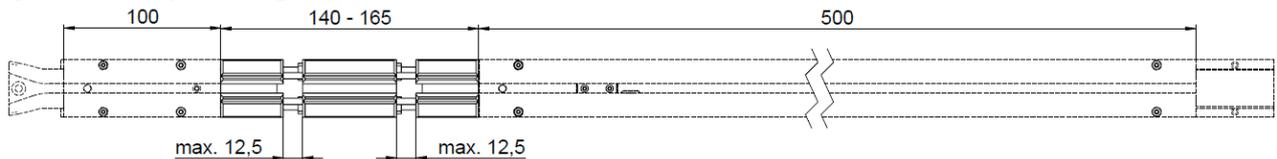
Fig. 65: Expansion unit – end feed (mounted on left)
