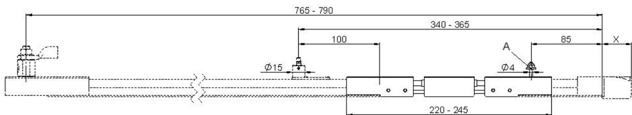
Fig. 68: Expansion unit – end feed (mounted on right), A = Anchor point
