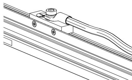
Fig. 96: PE connection is mounted
