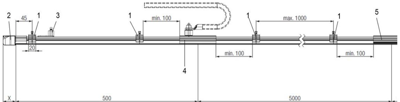
Fig. 33: Minimum and maximum distances between hanger clamps
