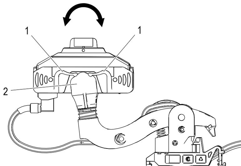
Fig. 188: Move collector head back and forth
