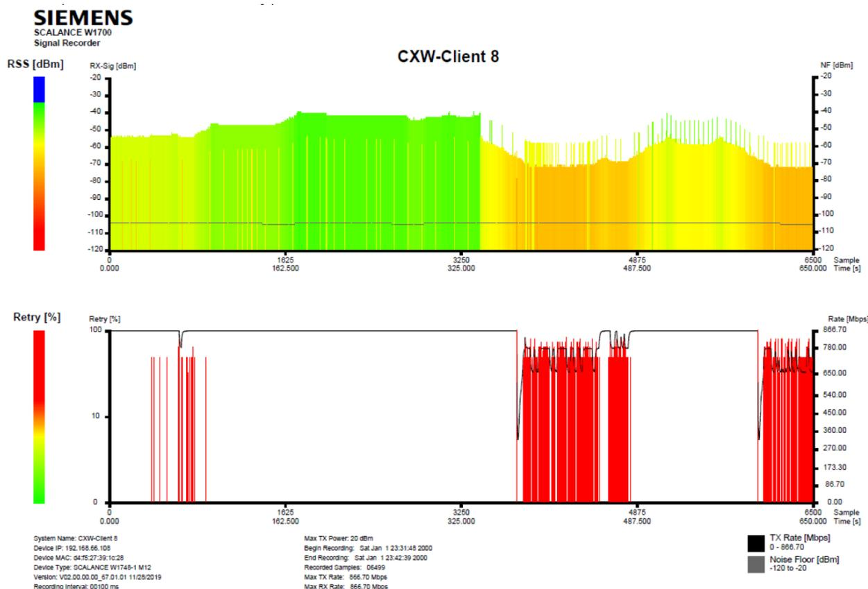
Fig. 204: Signal scan with too low signal strength, resulting in many retries and data rate drop
