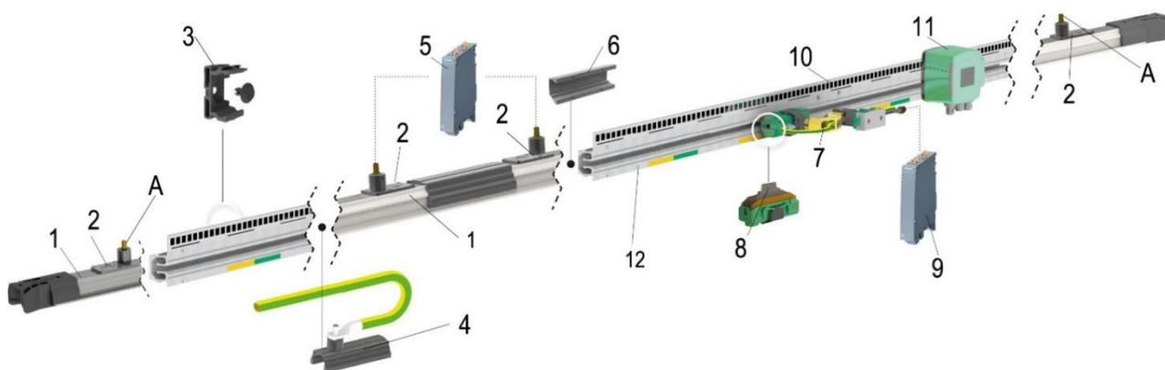
Fig. 15: ProfiDAT®compact components in detail
