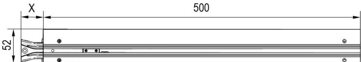
Fig. 44: Distance from rail edge to stationary antenna
