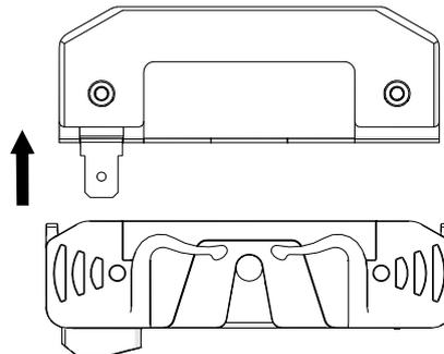
Fig. 159: Remove worn sliding contact
