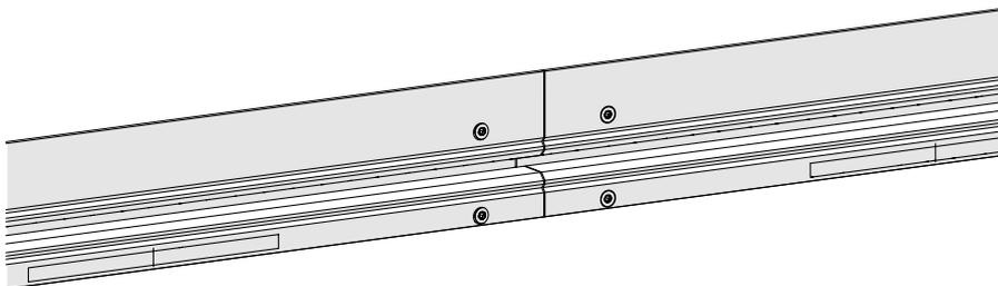
Fig. 81: Fully mounted connection point of rails without offset
