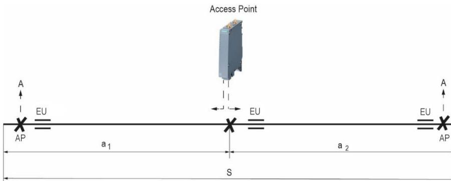
Fig. 50: Expansion unit dimensioning on segment
