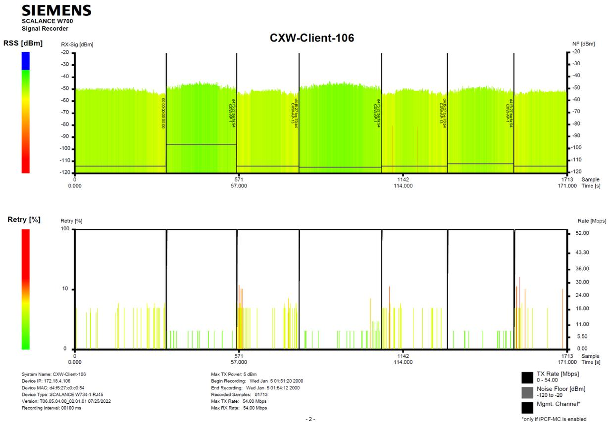
Fig. 201: Multiple crossing of same segment transfer with fault-free roaming operations (only single vertical black lines in transfer area)
