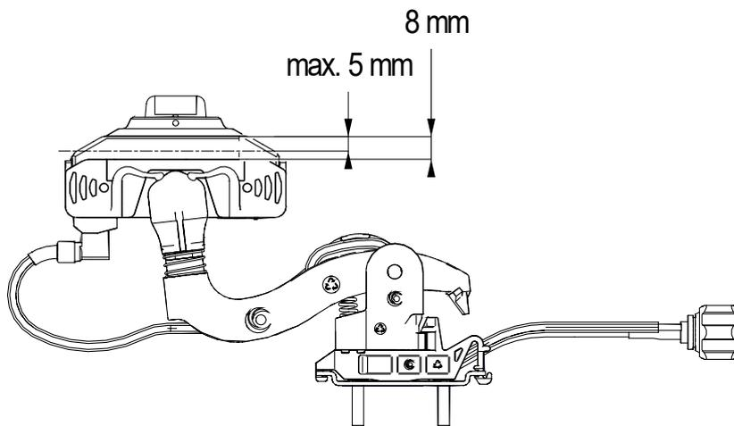
Fig. 146: Wear limit of sliding contacts on ProfiDAT®compact collector
