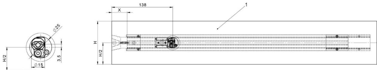
Fig. 47: Support structure (substructure) (1) with line feed (plastic cap, left)
