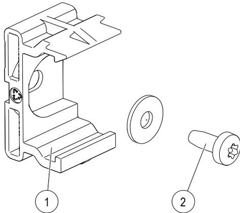
Fig. 37: Hanger clamp with self-tapping screw
