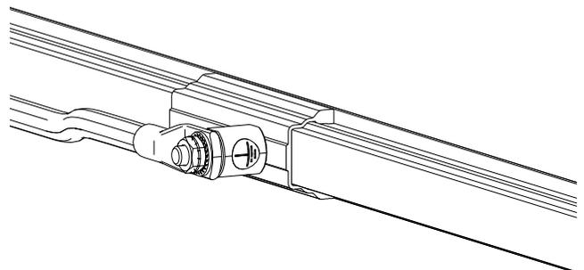
Fig. 93: PE connector is mounted
