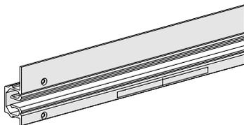
Fig. 17: Rail with positioning strip
