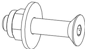
Fig. 60: Anchor point screw
