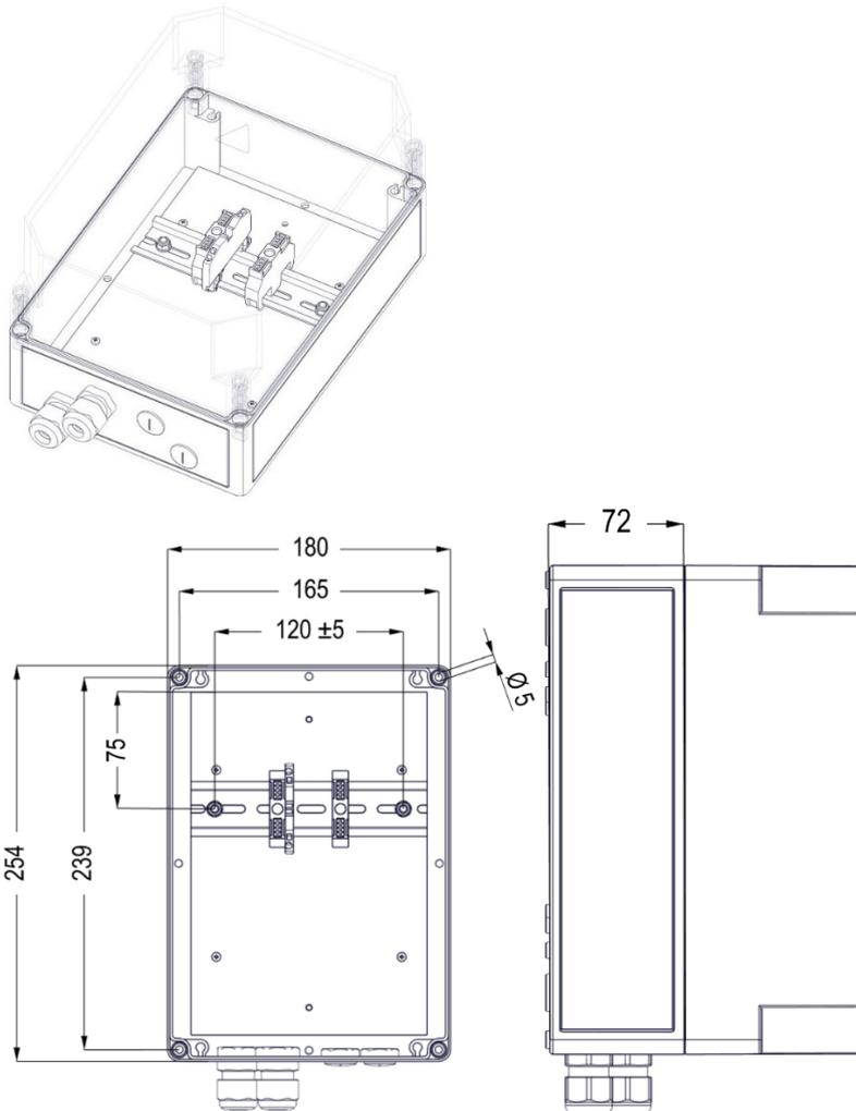
Fig. 4: Polycarbonate housing dimensions and illustration
