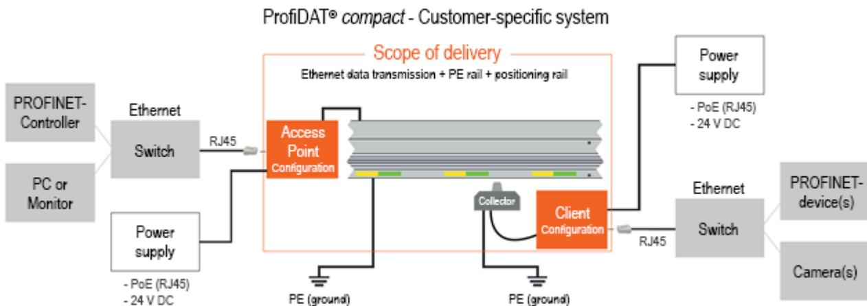
Fig. 1: Overview of interfaces and scope of delivery ProfiDAT<sup>®</sup>compact (simplified)
