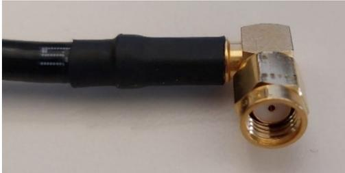
Fig. 5 R-SMA angle connector
