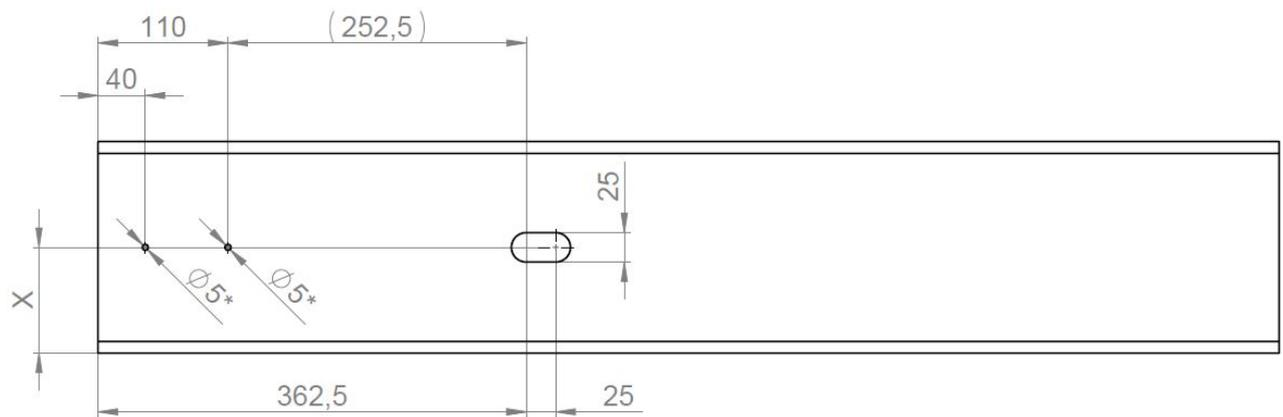
Fig. 120: Drill hole positions for end feed with expansion unit and aluminium overrun cap
