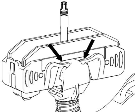
Fig. 165: Correct position of springs
