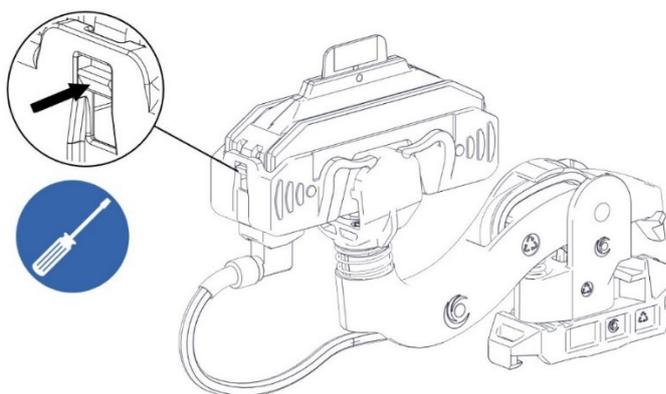
Fig. 173: Carefully press nose in collector housing inward with flat-head screwdriver
