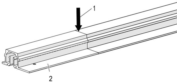
Fig. 97: Shorten ProfiDAT®compact rail (with positioning strip)
