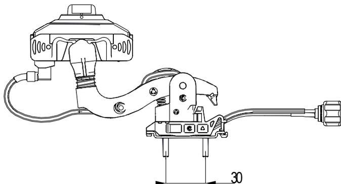
Fig. 126: Screw distances in towing unit
