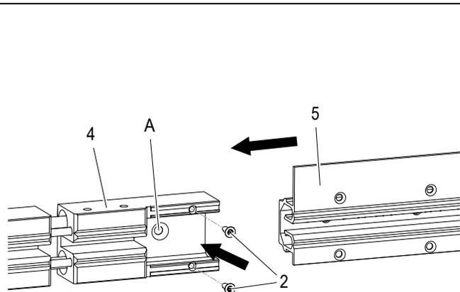
Fig. 63: Mount rail adapter
