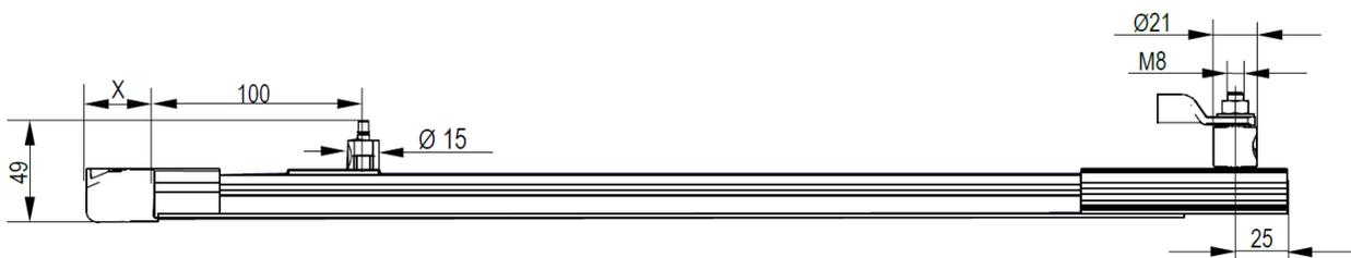
Fig. 45: Distance from rail edge to stationary antenna
