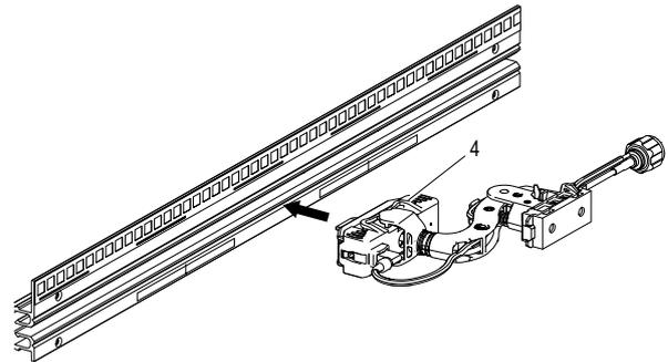
Fig. 125: Slide collector into rail
