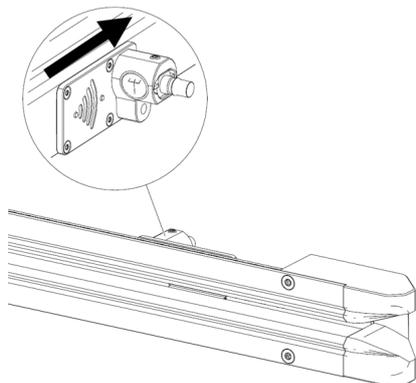
Fig. 25: End feed with stationary antenna
