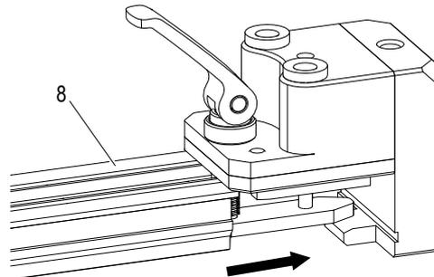
Fig. 107: Slide data rail (8) up to rail stop
