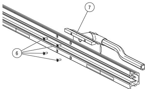
Fig. 92: Tighten all 4 self-tapping screws
