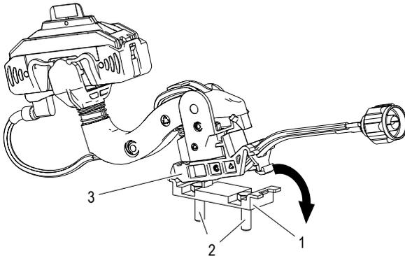
Fig. 124: Mount collector on towing unit
