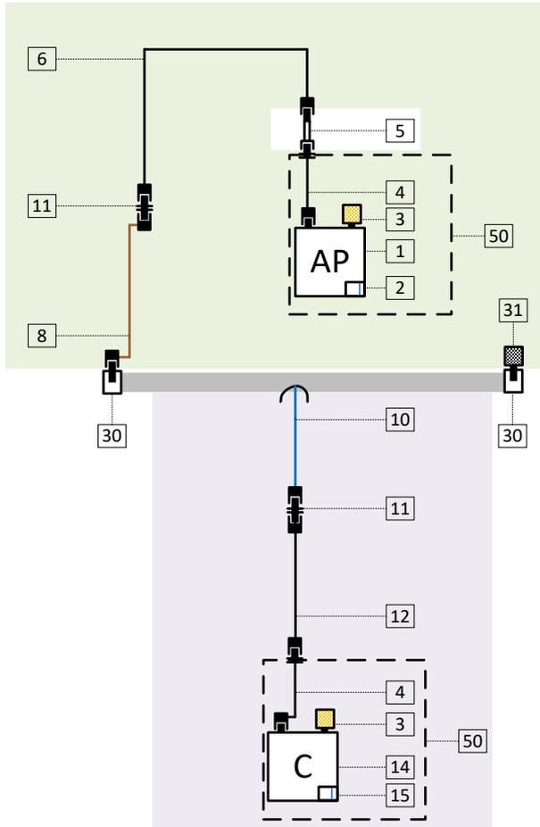
Fig. 30: Overview and arrangement of the electrical components. Example: End feed, client with one antenna, without additional housing, equipotential bonding not shown
