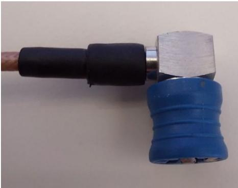
Fig. 6: QLS connector is unlocked
