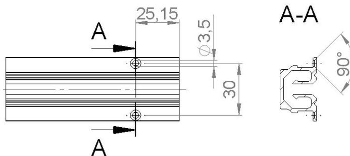
Fig. 114: Check distance dimensions
