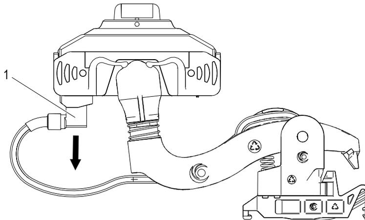
Fig. 170: Pull off angled blade receptacle
