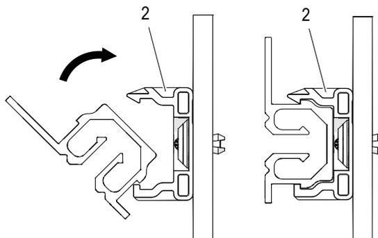
Fig. 76: Mount rail (from front)
